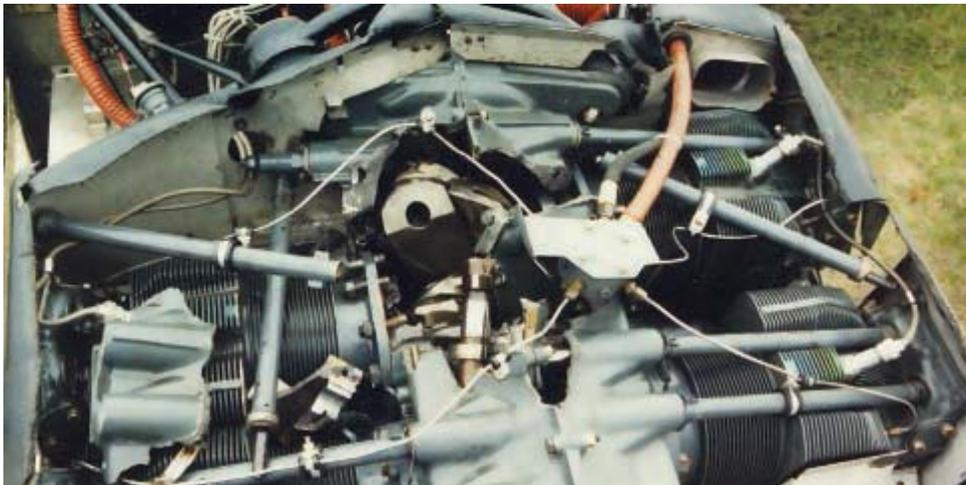
*This photo shows the aftermath of a crank shaft failure on an IO-360. After the engine failure, the pilot safely landed the plane in a nearby field. The cam shaft broke in half and the crankcase, as you can see, was ripped apart in flight.*
