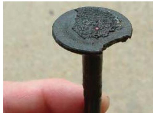
*Exhaust valves often don't survive to TBO. If we don't catch a potential exhaust valve failure using compression tests, borescope inspections, and engine monitor data, we risk a total failure ("swallowed valve").*
