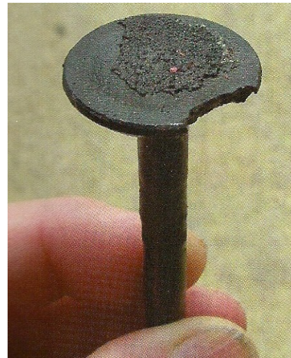
Figure 3 – Exhaust valves often don't survive to TBO. If we don't catch a potential exhaust valve failure using compression tests, borescope inspections, and engine monitor data, we risk a total failure ("swallowed valve")
